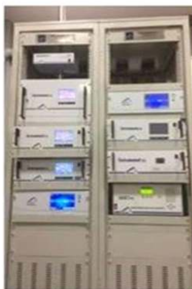
Front-view with data display of the AQMS and rack-mounted PM, Gas Analyzers and
